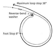
**Figure 5.** The maximum and minimum loop size for cable restraints is easily measured by circumference. The minimum loop stop is set at 8 inches and the maximum loop stop is set at 38 inches from the reverse-bend washer end of the cable. This results in a loop no smaller than 2½ inches in diameter and no larger than 12 inches in diameter.
