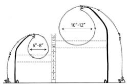
Figure 4. Loop heights and size vary depending on the intended species: coyote, bobcat or fox. Multiple swivels are recommended on a cable restraint. However, only a single swivel is required.
