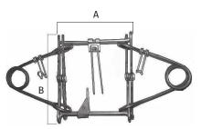
**Figure 1.** To determine the maximum square inches of an unset trap, multiply the maximum width of the trap jaws (A) by the height of the trap jaws (B). Body-grip trap designs vary.
